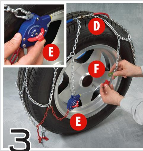
3. Grasp the top tensioner (E) and flip the red lever up to install. Pull the red cable end out and attach to the green side chain connector (F).
