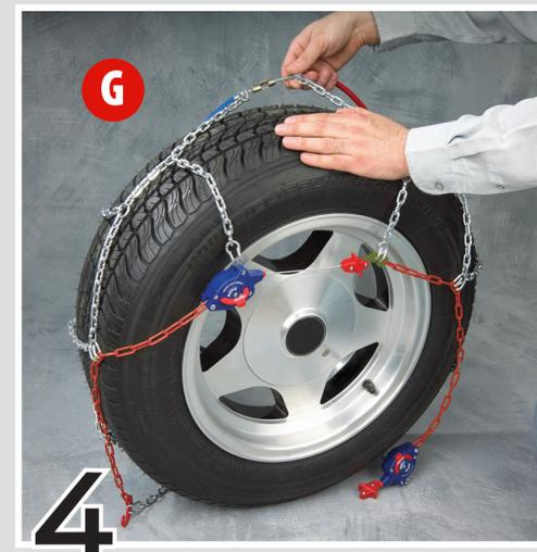
4. Leave the red lever in the up position and slide the side cable to the back of the tire (G), Ensure the chain is centered on the tire.
