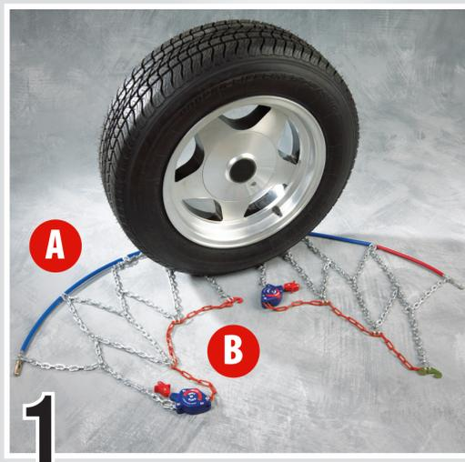
1. Lay the chains out on a flat surface, remove all tangles and ensure the wire hooks are facing down. **Do Not** drive with chains that are damaged.
