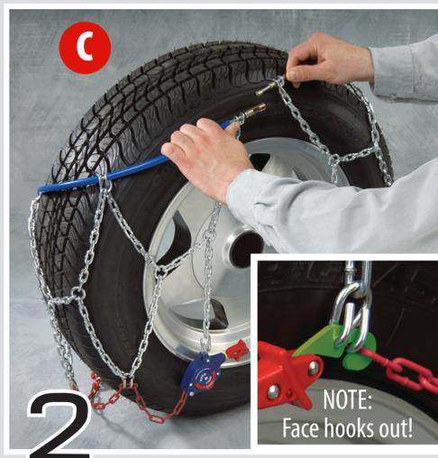
2. Bring the ends of the side cable in front of the outer side wall.
