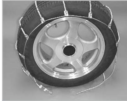
**2** Drape the chain over the tire so that the smooth side of the cross member hook is against the tire. The cross member nearest the end hook should touch the ground.
