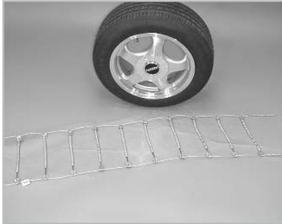
**1** Park vehicle on firm level ground, away from traffic and turn off the engine. Set the emergency brake. Chains should be installed on drive tires. Unroll the chain on the ground next to the tire. Position the cable so the end hooks are toward the front of the vehicle.
