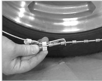
**5** Drive the vehicle one car length forward. Firmly tighten all connections. Use the clip on the side cable to secure the excess cable end. Note; the inside and outside connection should not differ by more than one metal bushing. See the close-up drawing below for a detailed look at this connection
