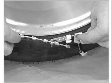
**3** At the inner sidewall, make the connection on the inside of the tire by pushing the cable with the end bushings behind the tire and toward the front of the vehicle.
