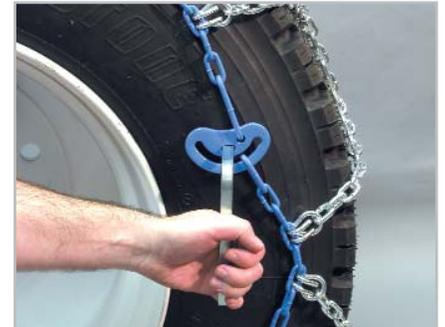
**6** Cam side chain adjusters should be closed by turning the cam clockwise with the included cam tightening tool. If there are more than 2 "loose" links at any of the fasteners, we recommend that you secure them to the side chain with a piece of wire or a plastic tie.
