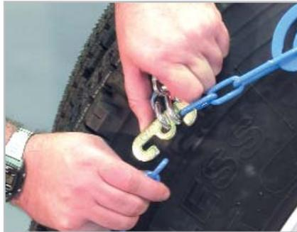
**5** Next fasten the outside fastener, again making sure it is as tight as possible. Drive a short distance and retighten all fasteners. For best results, make sure fasteners are adjusted equally and as tight as possible.
