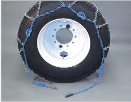
**1** Park vehicle on firm level ground and turn off the engine. Set the parking brake. Lay the chains out flat on the ground, making sure there are no twists or tangles. Make sure the cross chain hooks are facing upward, then drape chain over the tire, so that one cross chain is positioned at the point where the tire meets the ground.
