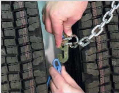
**4** Reach behind the tire and fasten the inside connector making sure it is as tight as possible.
