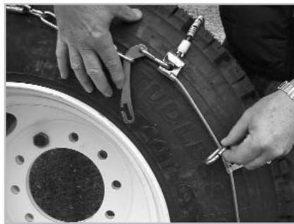
**5** Fasten the outside connector by passing the long lever through one of the chain links, folding it back in the opposite direction and securing the "keeper" link on the end of the lever. If care is taken to make this connection as tight as possible, it may not be necessary to retighten after driving. If you find that the inside fastener also has to be adjusted to assure a snug fit, you should do it before fastening the outer fastener.
