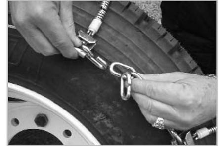
**3** Connect the "speed hook" on the inside of the tire (the side away from you). As a starting point, we recommend that you fasten it so that there are no more than two "free" links. It may be necessary to drive forward two to three feet so that the inside connection can be made more easily.
