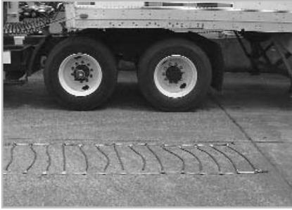
**1** Park vehicle on firm level ground, away from traffic. Unroll the set and lay each half pair on the ground next to the tires it is intended to cover. Make sure that there are no twists or kinks in the cable chain. Make sure that the smooth side of the eyelets (marked "TIRE SIDE") will be against the tire. If the smooth side will not be toward the tire, damage will occur.
