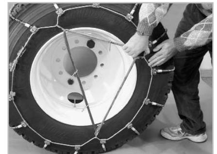
**6** Install the rubber tightener. Always stretching the tightener from one hook to the next farthest from it. Make sure that the tightener hooks are facing away from the tire. If hooks are not facing away from the tire, damage will occur. Chain may now be driven without further adjustment.
