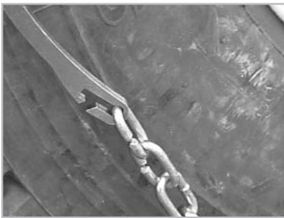
**4** Connect the outside fastener at its loosest setting, then pull the cable towards you to create as much slack as possible. Make sure that none of the cross members are caught in the "shoulder" area of the tire tread.
